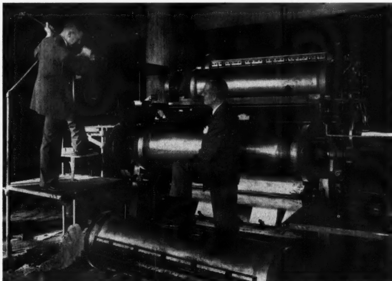
J. Louis Landenberger, president of Ketterlinus Litho Mfg. Co., Primos, Pa., wields a sledge hammer on a 44x64-inch two-color Harris offset, which the company purchased new in 1929. The old machine was still producing good work, but production was not high enough to compete with newer presses. Replacing it is new 50x72-inch press. Watching is Ralph Randall of Harris-Seybold
